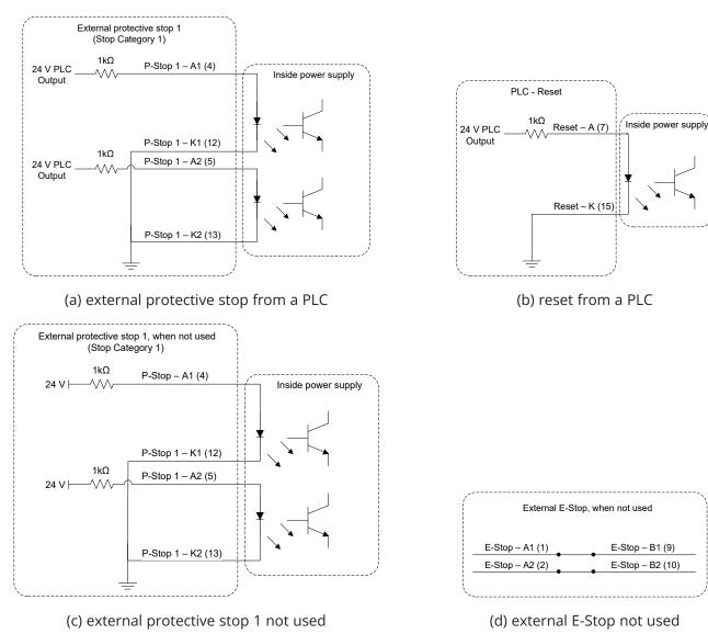
Figure 23: Additional examples of connections to D-SUB connector (resistances are mandatory in R3)
