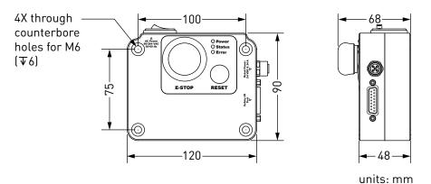
Figure 9: Dimensions of the Meca500 intelligent power supply
