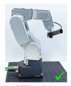
(a) DO NOT leave the robot deactivated like this (b) DO leave it like this Figure 5: Before leaving the robot deactivated for an extended period of time, move it to a position that minimizes the static joint torques
