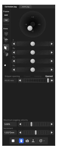
(b) Cartesian jogging using the secondary mouse button Figure 17: Cartesian jog tab
