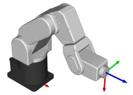
Figure 19: Robot position when the TRF is at x = 250 mm, y = 0 mm, z = 150 mm,  $\alpha = 0^{\circ}$ ,  $\beta = 90^{\circ}$ ,  $\gamma = 0^{\circ}$  with respect to the WRF
