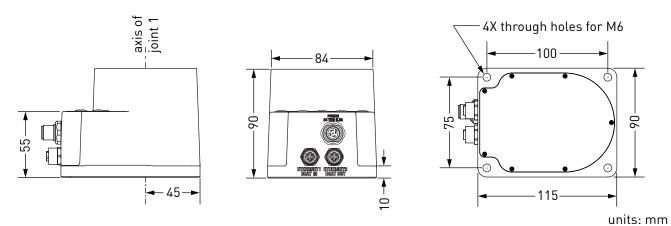
Figure 7: Dimensions of the robot base
