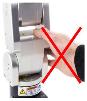
Figure 1: Pinch point example
