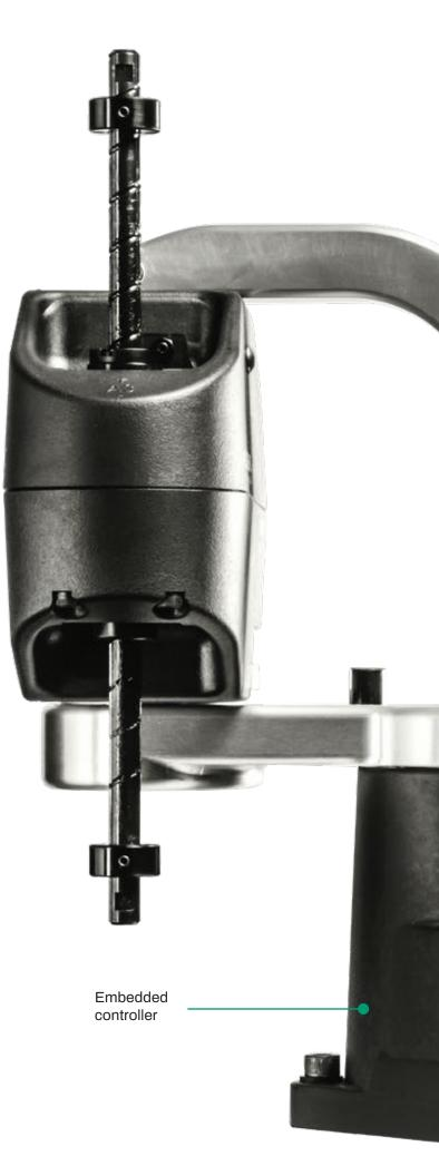
Rated payload is 500 g. Max. payload is 1 kg, under certain conditions.
